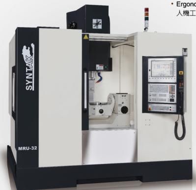
Syntak 5-axis machining center MRU Series is for producing high accuracy components. The integrated 4th and 5th rotary table allows complicated or multiple faces parts to be machined in just one setup. In addition, with the unique dual lead worm shaft and the hydraulic braking system, the rotary table features high power transmission rate, which meets all technical demand for heavy duty cutting.
