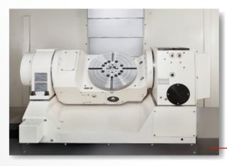
The Dual-axis rotary table on Syntak MRU Series machine features C axis 0.001° indexing resolution and wide tiling range of A axis (-120° to +30°), suitable for various complex surface or multiple face machining.
